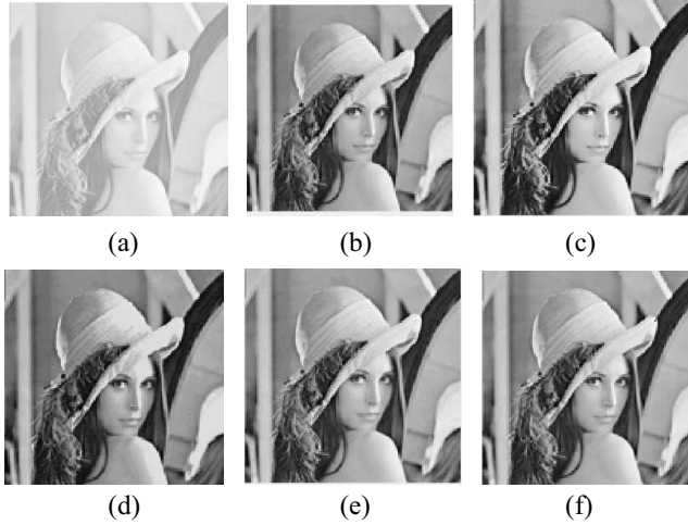
Fig. 12. Example of the original image and contrast stretch results operated by various dividers. (a) Original image. (b) Fixed-point divider. (c) ISCBDIV. (d) DFSMDIV. (e) CBDIV. (f) FSCDIV.
