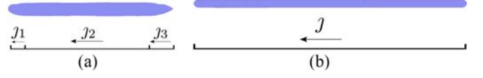
Fig. 8. Wires with irregular shape due to the lithography process [23]. (a) Short wire. (b) Long wire.
