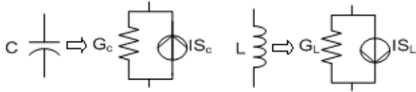
Fig. 5 Linear Model of L and C Component
