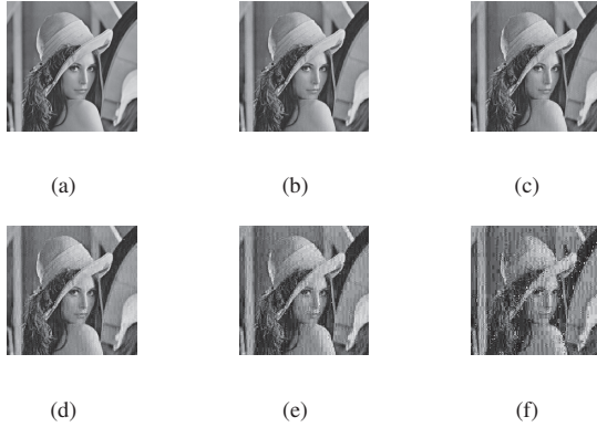
Fig. 4: (a) The initial image before DCT/IDCT process; (b) Image after DCT/IDCT process using 10-bit stochastic multiplication; (c) 9-bit; (d) 8-bit; (e) 7-bit; (f) 6-bit.
