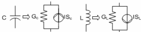
Fig.2. Linear Model of L and C Components.
